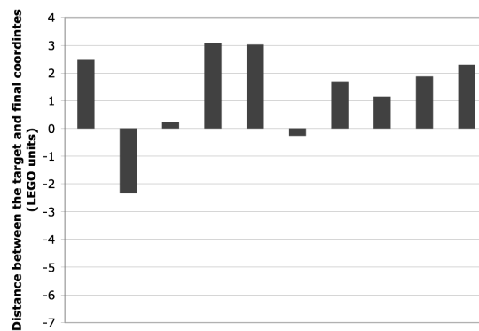
Figure 2 Results of the targeting accuracy tests of the LEGO robot. In each graph, the x-axis shows the results from each of the ten targets. The y-axis shows the distance between the target coordinate and the final needle position in the x, y and z directions for figures A, B and C, respectively.
