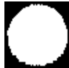
Figure 1: Approximate circular structuring element, radius 25, constructed using 8 lines.
